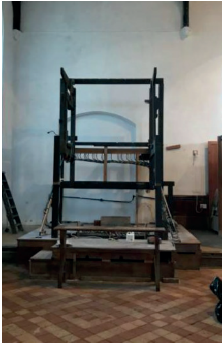
The building frame - bereft of all pipes, chests and action.
