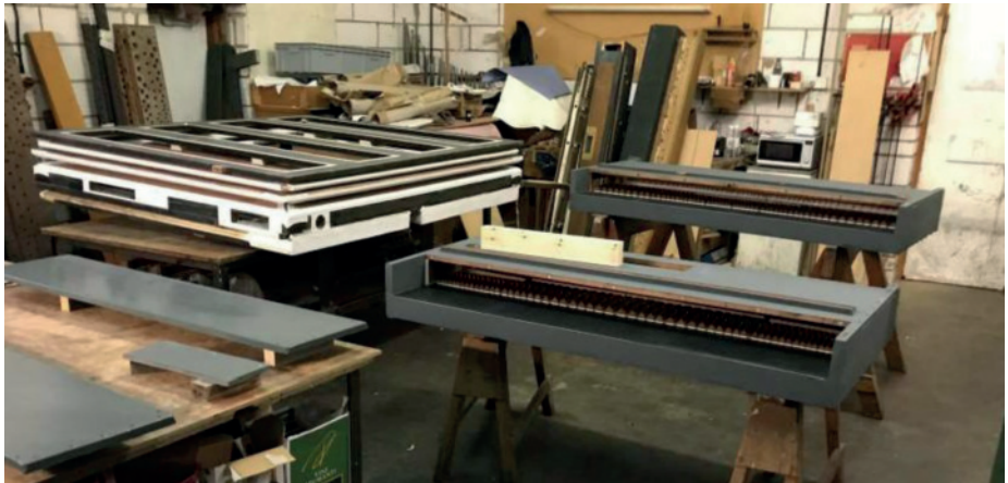
The reservoir, Great and Swell windchests in the Weston Longville workshop after restoration.
